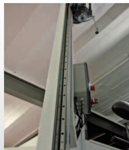
Detail of photocells curtain.
