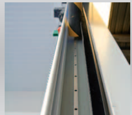
Detail of infra-red barrier.
